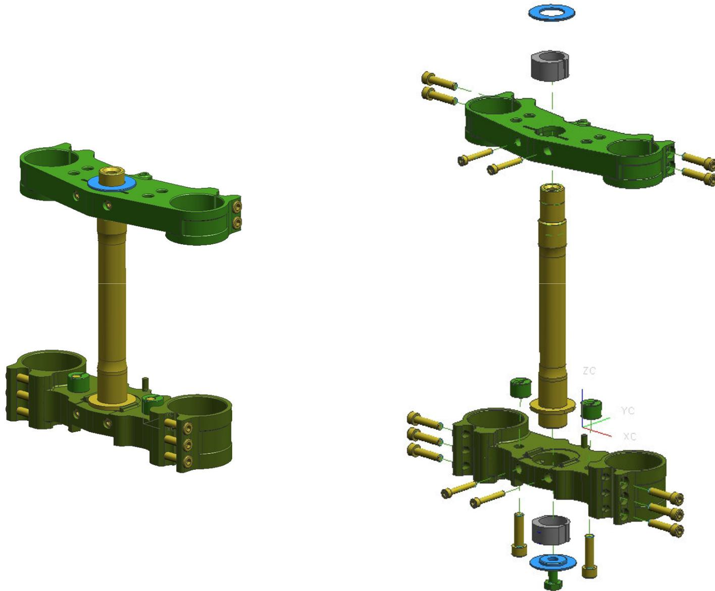
CAD (Computer Aided Design) – Disegno 3D 'ASSEMBLATO' ed 'ESPLOSO'
