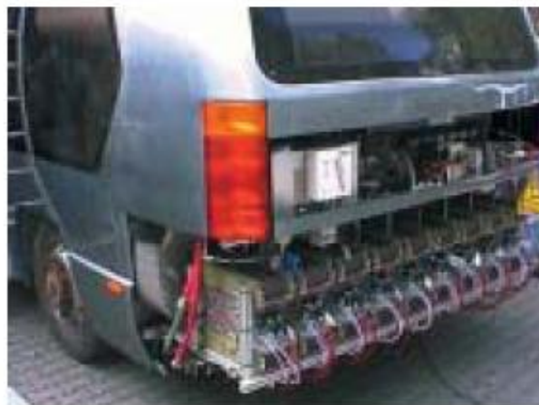
A hydrogen fuel cell engine in the rear of a bus.
