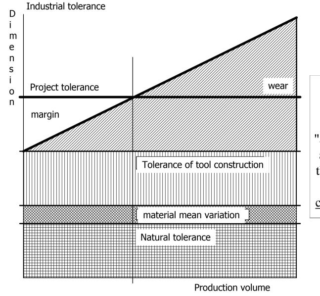
In the definition phase of industrial tolerance the components "natural tolerance", "average variation of the material" and "tolerance of construction of the tool" shall be considered to be <u>constant in relation to the</u> <u>cumulative volume of production</u>.
