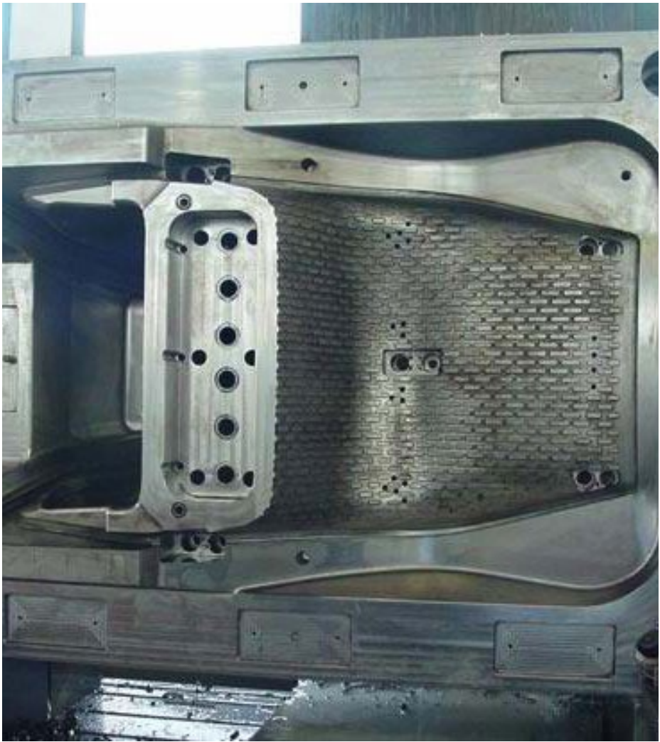
MYTO CHAIR 3. MOULD IN STEEL FABRICATION
