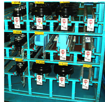
Parts Shelf with Fool Proof System Parts Shelf with Selection Lamp ・ポカヨケ付き部品棚 ・仕様指示ランプ付き部品棚
