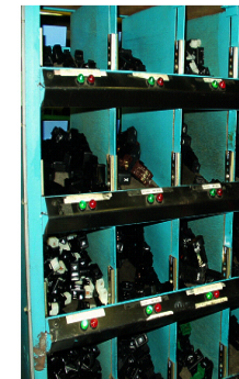
Parts Shelf with Fool Proof System Parts Shelf with Selection Lamp ・ポカヨケ付き部品棚 ・仕様指示ランプ付き部品棚
