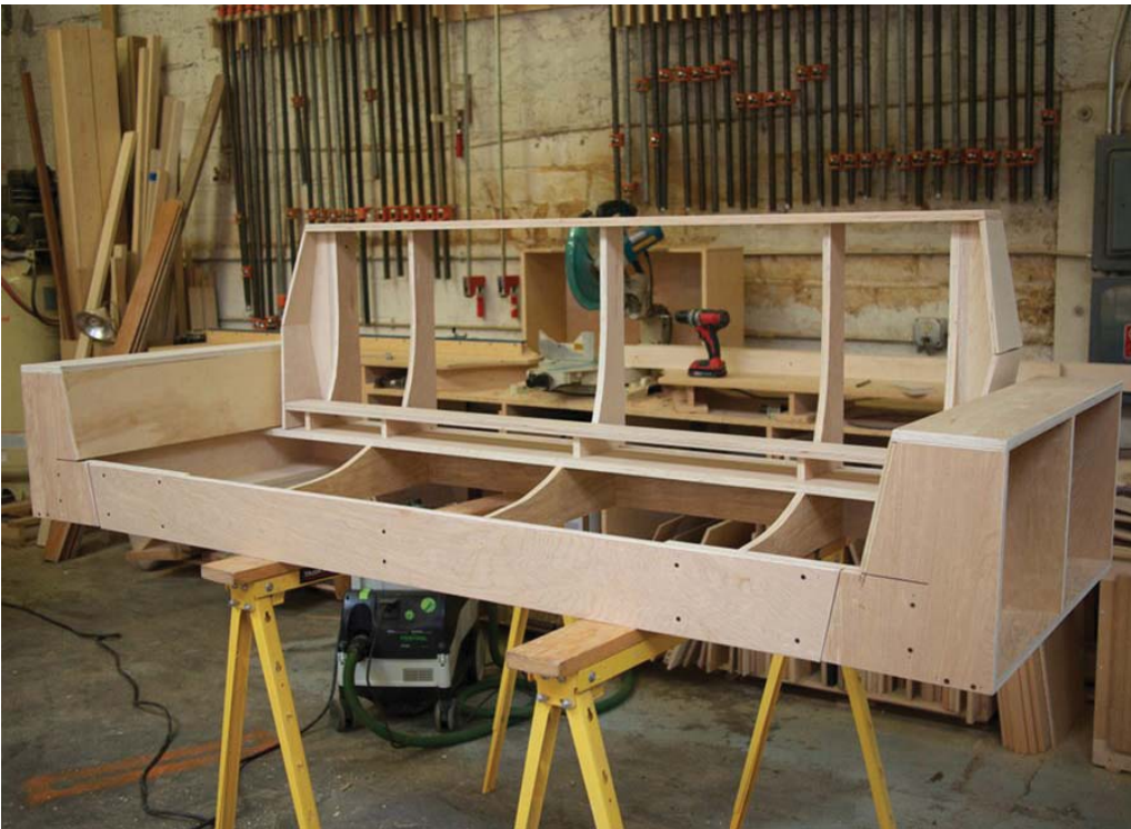
1. WOODEN FRAME CONSTRUCTION
