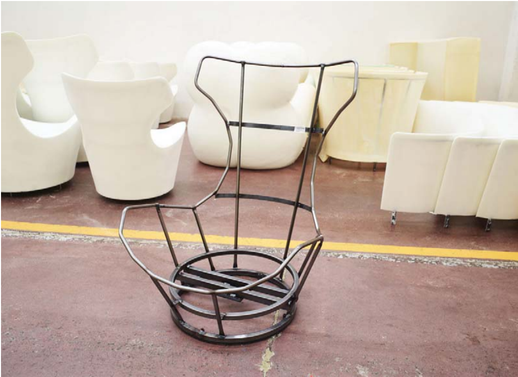
GRANDE PAPILIO ARMCHAIR 1. METAL FRAME INSERT
