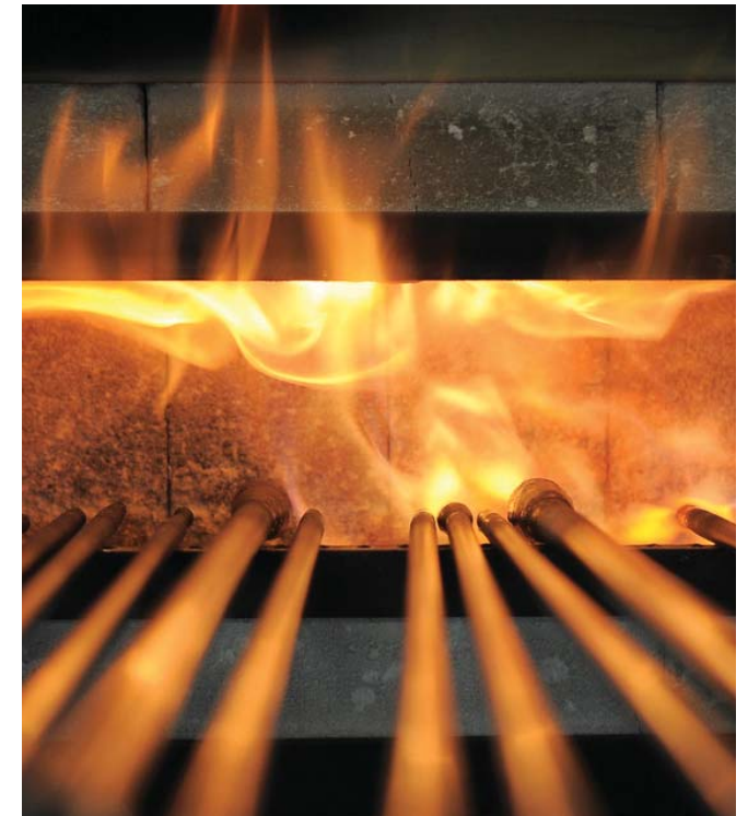
3. BLOW PIPE COLLECTING MELTED GLASS
