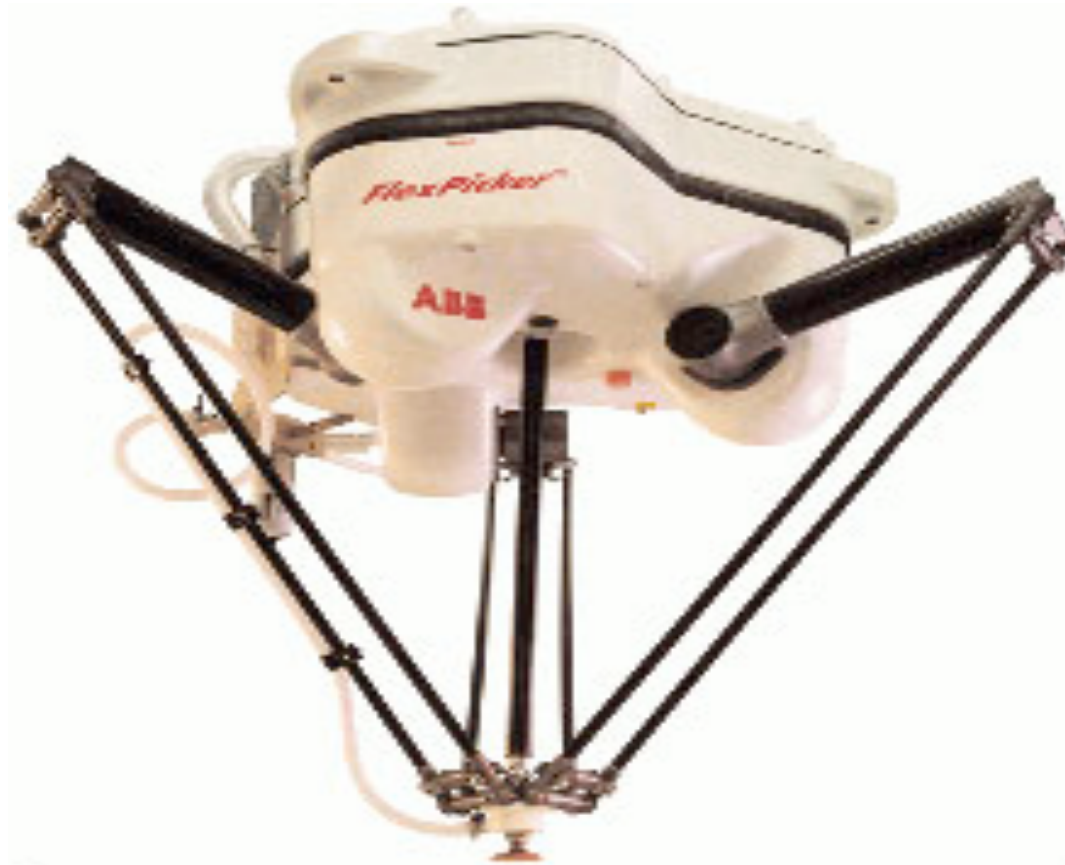
ABB Flexible Automation's IRB 340 FlexPicker (courtesy of ABB Flexible Automation) ... from http://www.parallemic.org/Reviews/Review002.html
