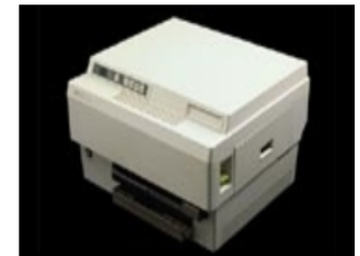
The HP LaserJet was the world's first desktop laser printer.
