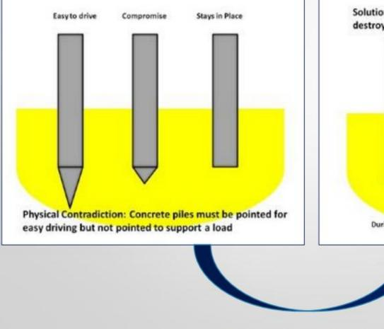
Solution: The piles are made with pointed tips which are destroyed after driving, via an embedded explosive
