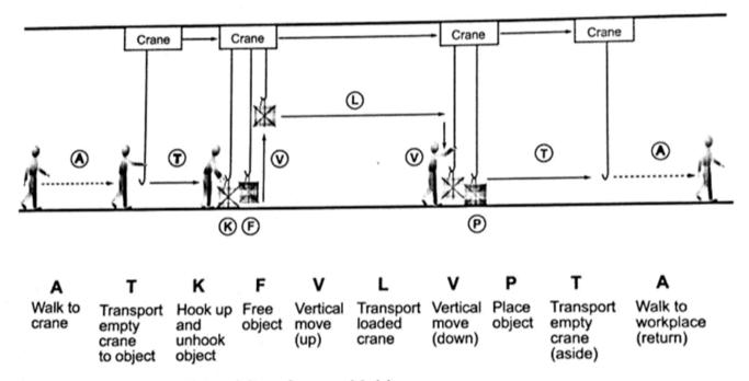
Figure 3.55 Illustration of Manual Crane Sequence Model.
